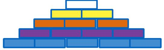
Figure 14 A shift-invariant, scalable operator. Processing is from the bottom (input) to the top (output). Each layer consists of identical blocks, each block has two inputs and one output; each block is an operator  $H_2 : \mathbb{R}^2 \mapsto \mathbb{R}$ . The step of combining two inputs to a block into one output corresponds to coarse-graining of a Ising model.
